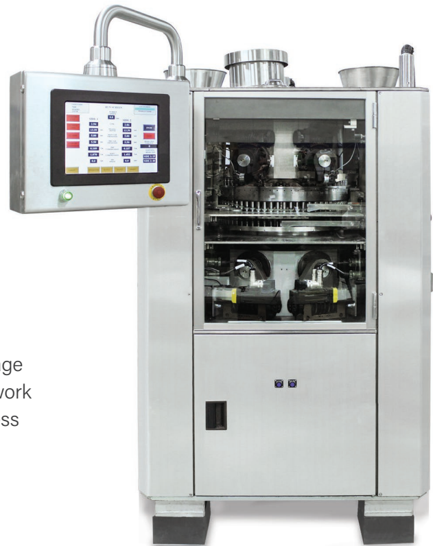
Reconditioned Kikusui press with enhanced control system.
